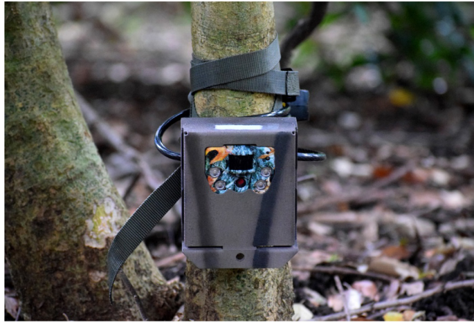
Fig. 3. A camera trap attached to a tree trunk to capture images/videos of Indian pangolins.
