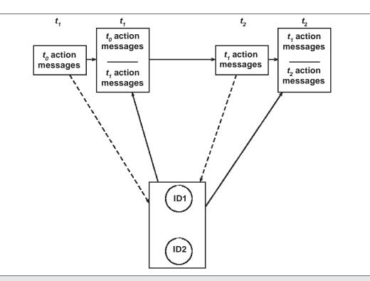
Fig. 2. Sequential updating scheme of an IntIDs model consisting of two IDs. Bulletin board states are indicated by the boxes in the top row. A dashed arrow indicates messages are read but not removed. A solid arrow indicates message addition.
